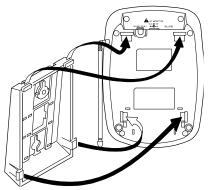
2. Plug one end of the supplied short modular cord into the TEL LINE jack on the back of the base.
